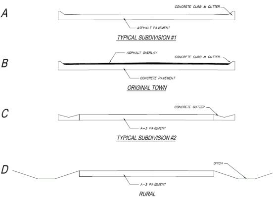
Section 3.21 Typical Existing Roadway Cross Sections
